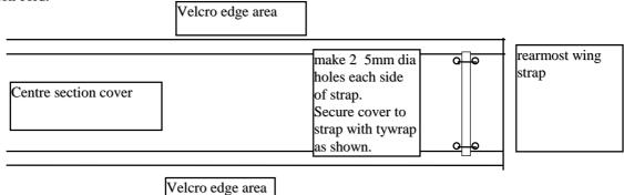
New gap covers are now supplied with straps to additionally secure the cover to the centre section straps (Cyclone Airsports minor modification AX268).
