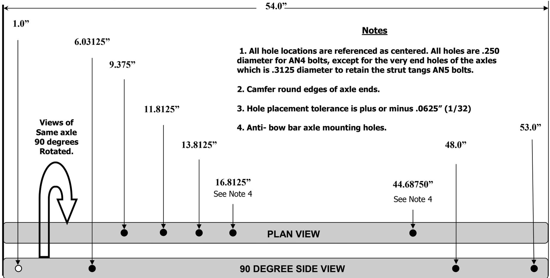
Axle has a finished overall length of 54." It is a length of 6061T6 Aluminum 1.0" O.D. solid bar round stock and weighs 4.0 lbs when finished to install. Not recommended for aircraft whose pilots weigh more than 170 lbs., because it will bend. Use a steel axle for heavier pilots.
