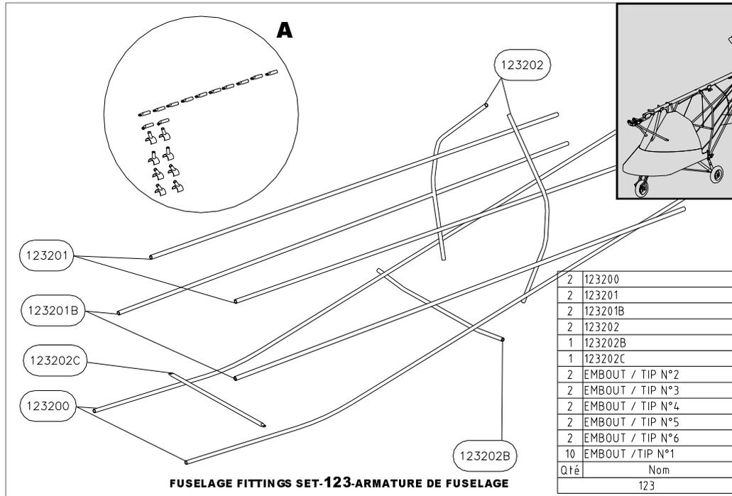
FUSELAGE FITTINGS SET-123-ARMATURE DE FUSELAGE
